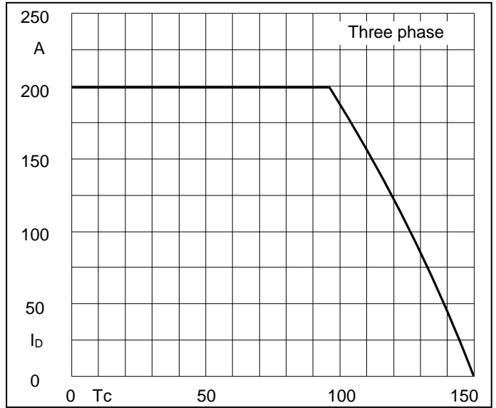
Fig2. Forward Current Derating Curve
