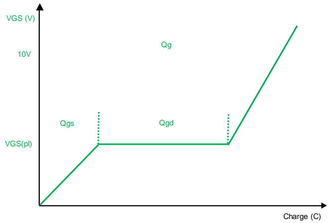
Figure B. Gate Charge Test Circuit & Waveform
